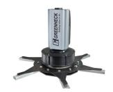
Lightweight, direct drive motor is up to 20% more efficient and 10 dBA quieter than traditional gearbox motors. Factory-mounted and programmed VFD reduces installation time by eliminating complicated programming in the field.
