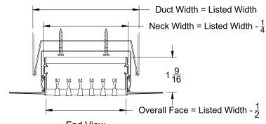
**End View** Duct Length = Listed Length -Neck Length = Listed Length -  $\frac{1}{4}$ Overall Length = Listed Length +  $2\frac{3}{4}$
