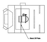
Titus® HD,TDH,TDH,TSH, LD, HS Series Replace all mechanical regulators with combination of flanged retrofit assembly(ies) and blank off plate(s) through bottom access panel. One actuator per valve, field or factory mounts on valve body. Flow controller panel is mounted in the field on outside of HD air terminal casing.
