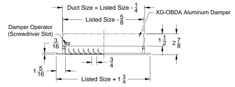
Option: XG-EPRHDP-1 (Engineered Polymer Register - with Polymer Damper - 45° Fixed Blades)
