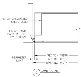
NOTE: ADDITIONAL STRUCTURAL REINFORCING MEMBERS MAY BE REQUIRED (BY OTHERS) TO SUPPORT AND INSTALL MULTIPLE LOUVER PANELS WITHIN A LARGER OPENING.
