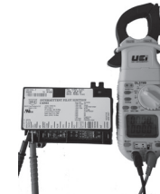
Fig. 3 BASO Ignition Control
