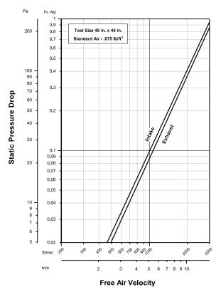
Louver Type AC153 resistance to airflow (pressure drop) varies depending on louver application (air intake or air exhaust). Free area velocities (shown) are higher than average velocity through the overall louver size.
