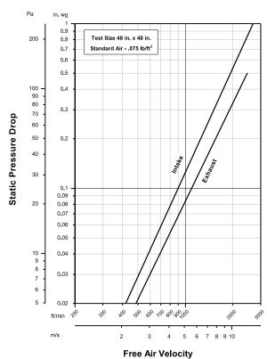
Louver Type AC154 resistance to airflow (pressure drop) varies depending on louver application (air intake or air exhaust). Free area velocities (shown) are higher than average velocity through the overall louver size.
