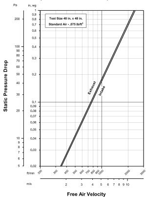
Louver Type AC155 resistance to airflow (pressure drop) varies depending on louver application (air intake or air exhaust). Free area velocities (shown) are higher than average velocity through the overall louver size.
