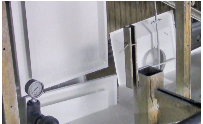
Diffusers exiting paint tank with white finish.
