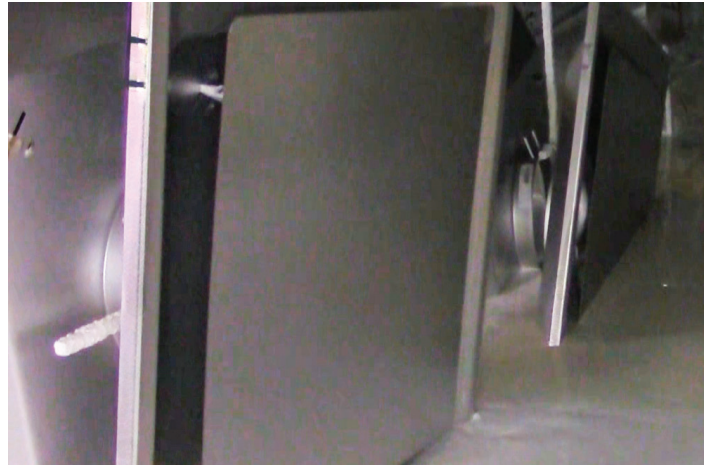
Diffusers being submerged in paint tank.
