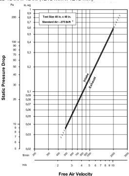
Model K6746HP resistance to airflow (pressure drop) varies depending on louver application (air intake or air exhaust). Free area velocities (shown) are higher than average velocity through the overall louver size. See louver selection information. (Test Figure 5.5-6.5)
