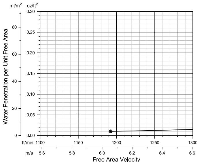
The AMCA Water Penetration Test provides a method for comparing various louver models and designs as to their efficiency in resisting the penetration of rainfall under specific laboratory test conditions. The beginning point of water penetration is defined as that velocity where the water penetration curve projects through 0.01 oz. (3 g) of water (penetration) per sq. ft. (m<sup>2</sup>) of louver free area.
