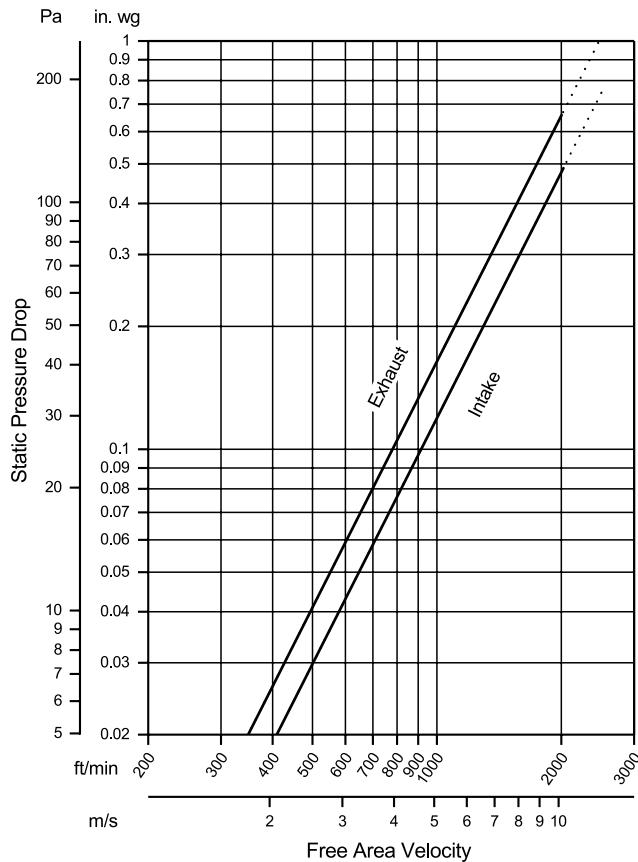
Model K8204E resistance to airflow (pressure drop) varies depending on louver application (air intake or air exhaust). Free area velocities (shown) are higher than average velocity through the overall louver size. See louver selection information. (Test Figure 5.5-6.5)
