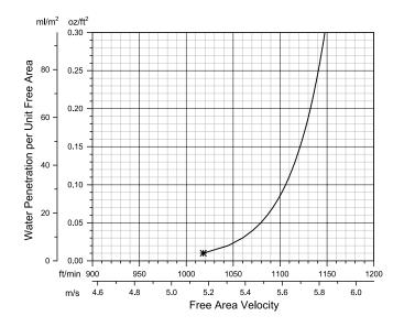
The AMCA Water Penetration Test provides a method for comparing various louver models and designs as to their efficiency in resisting the penetration of rainfall under specific laboratory test conditions. The beginning point of water penetration is defined as that velocity where the water penetration curve projects through 0.01 oz. (3 g) of water (penetration) per sq. ft. (m²) of louver free area.
