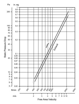
Model K8504 resistance to airflow (pressure drop) varies depending on louver application (air intake or air exhaust). Free area velocities (shown) are higher than average velocity through the overall louver size. See louver selection information. (Test Figure 5.5-6.5)
