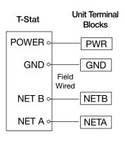
Note: Additional T-Stats should be daisy chained - do not make home runs back to the unit's terminal block nor the main controller.
