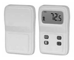
The space thermostat gives users the ability to view the space temperature and control the active space setpoints from the adjustable display. The space thermostat also has the ability to send the unit into temporary occupied mode. Up to four space thermostats can be wired back to the microprocessor to provide an average for the space temperature. The space thermostat is shipped loose with installation by others and is a Modbus connected device.
