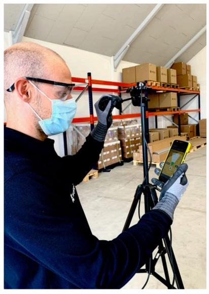
Measurement of irradiation in grid points.
