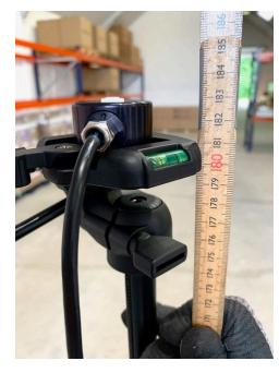
Setting the height of the sensor head to a standard 6 ft. (183 cm) or acceptable height for the tasks that are performed in the room.
