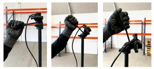
Examples of different sensor directions when measuring to locate hotspots.
