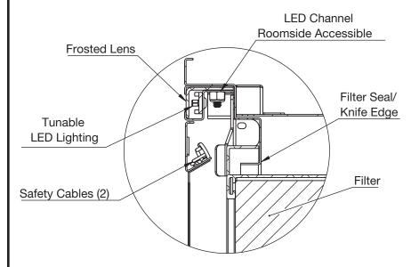
LED Lighting – Tunable and Dimmable White: 2700K – 6500K; Green: 525nm 2 LED light strips per unit
