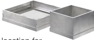
**Duct Adapters** - Duct adapters fit over the roof curb and support the top of the duct allowing ductwork to be completed before the fan is set in place. Duct adapters also limit performance losses by directing airflow into the duct.
