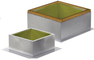
**Curb Extension** - Extensions raise the fan discharge above the roofline and provide an accessible mounting location for dampers. Insect screen bases are constructed with a removable fine mesh and recommended for applications where insect entry must be prevented.
