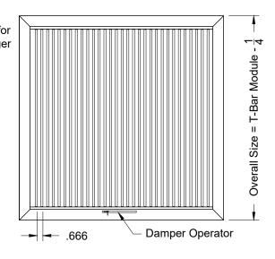
Note: This product complies with NFPA 90A-18 standard 4.3.7.3.2 and 4.3.8.3.2 and is constructed with openings through which a 1/2" sphere can not pass.
