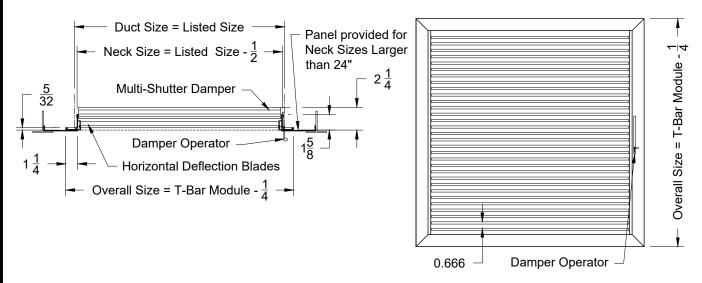
Note: This product complies with NFPA 90A-18 standard 4.3.7.3.2 and 4.3.8.3.2 and is constructed with openings through which a 1/2" sphere can not pass.
