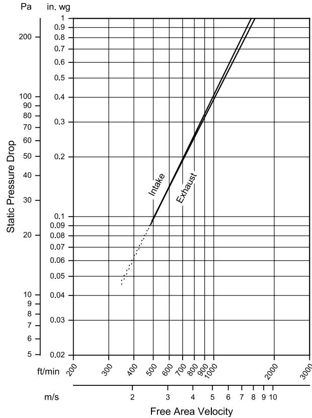
Model AFL-601 recessed/flush frame resistance to airflow (pressure drop) varies depending on louver application (air intake or air exhaust). Free area velocities (shown) are higher than average velocity through the overall louver size. See louver selection information. (Test Figure 5.5-6.5)
