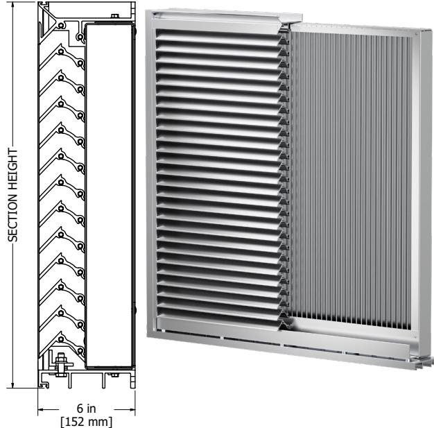
The AFL-601 is a UL Classified Wind-Storm Rated Assembly in accordance with FEMA Guidelines P-320 and P-361, and ICC 500 (2020 & 2023) to static and cyclical design pressures of positive/negative 350 PSF and debris impact of a 15 lb sawn lumber 2x4 traveling at 100 MPH (6.8 kg at 44.7 m/s).
