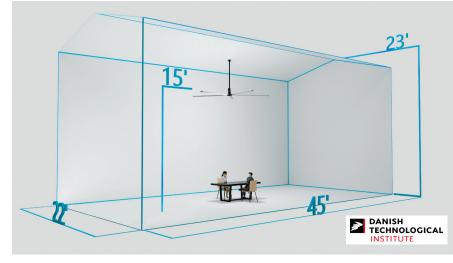
A single 10 ft. diameter fan was operated in a large room (dimensions shown to the right) with a high concentration of aerosolized MS2 virus.
