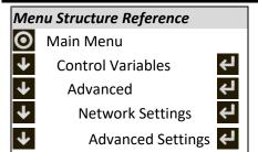
Additional settings can be accessed in the BACnet Advanced Settings menu including BACnet Broadcast Management Device (BBMD) configuration, relinquish default settings, Change of Value (COV) increments and restoring binary text values.
